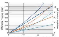
Flow rate (L/min), water at 20 °C per 254mm (10 in.) Module For liquids other than water, multiply differential pressure by fluid viscosity (cP).
